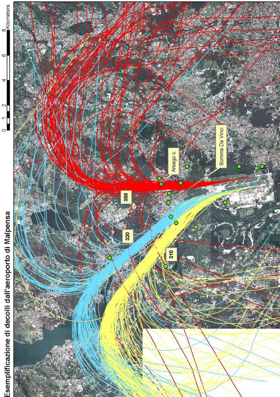
Figure 17: Takeoff tracks from Malpensa Airp.: yellow is 310, cyan is 320 and red is 358 SID.
