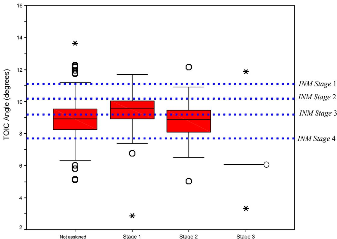
**Figure 4: Trajectory statistical distribution in the first climbing segment, case MD82, with INM *stage* assignment formulation. Blue dashed lines define INM values.**
