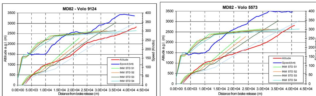
Figure 5: Speed (blue) and climbing profile (red) trend compared with INM procedural profiles.
