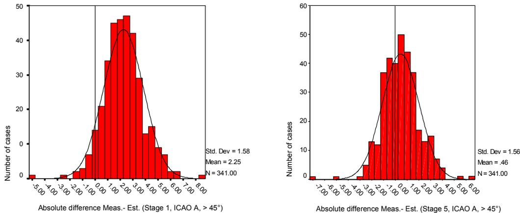
**Figure 15: Measured and estimated SEL differences distribution, comparison between stage 1 and stage 5 for ICAO A profile and  $\beta$  angle major than  $45^\circ$**
