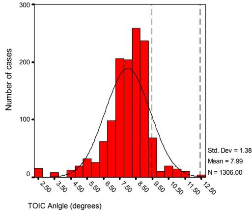
**Figure 6: Take Off Initial Climb angle distribution in A320 case; dashed vertical lines define values corresponding to INM stage 1 and stage 5.**
