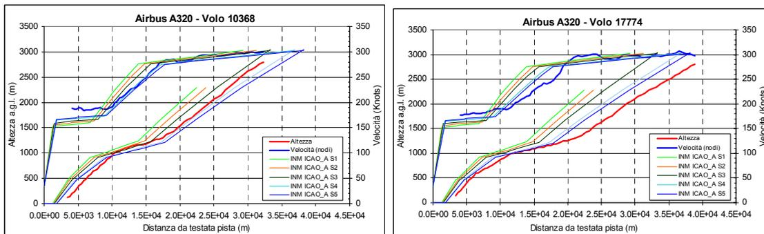
**Figure 7: Speed (blue) and climbing profile (red) trend compared with INM procedural profiles.**
