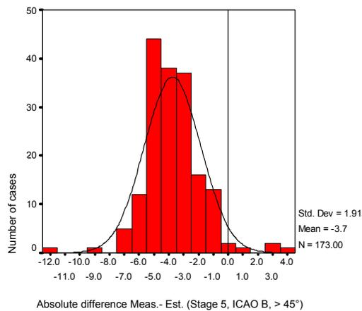
**Figure 16: Measured and estimated SEL differences distribution, comparison between stage 1 and stage 5 for ICAO B profile and  $\beta$  angle major than  $45^\circ$**
