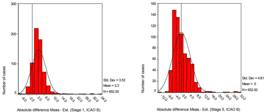
**Figure 14: Measured and estimated SEL differences distribution, comparison between stage 1 and stage 5 for ICAO B profile.**
