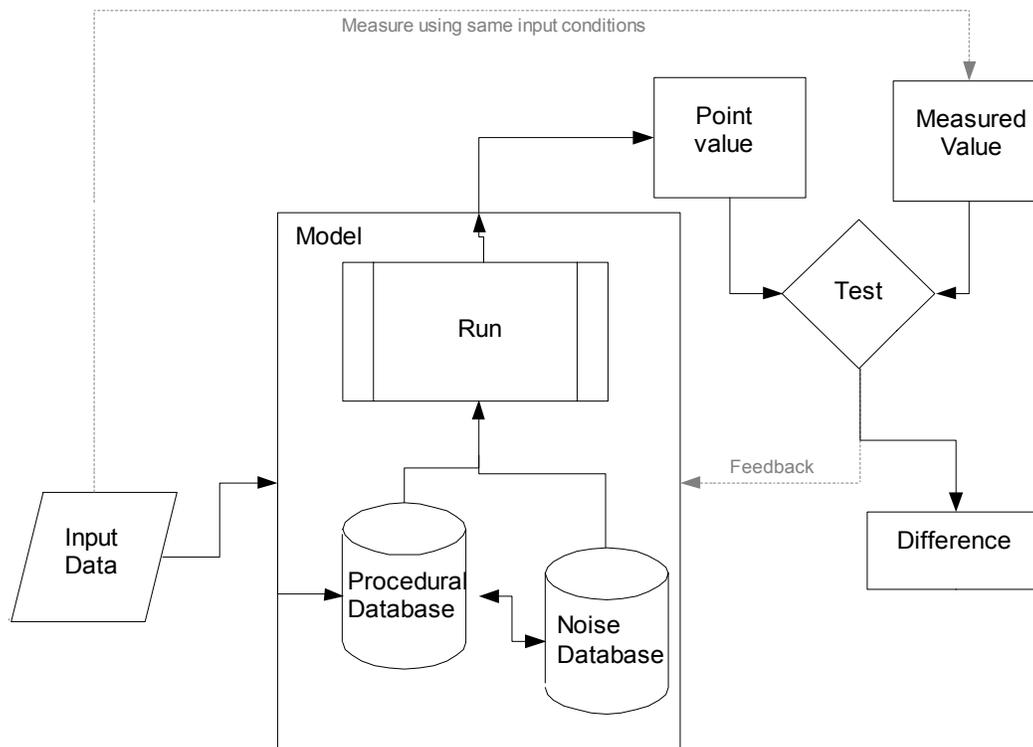
**Figure 1: difference evaluation procedure (validation) for a noise statistical model.**
