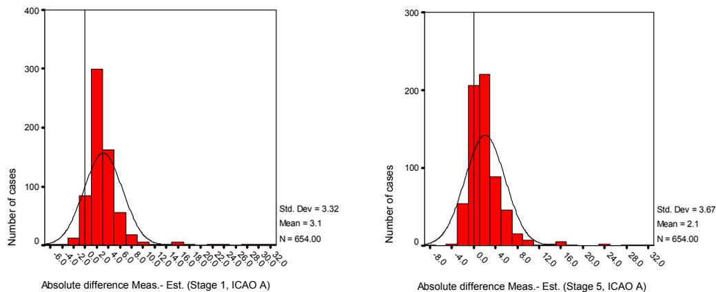
**Figure 13: Measured and estimated SEL differences distribution, comparison between stage 1 and stage 5 for ICAO A profile.**
