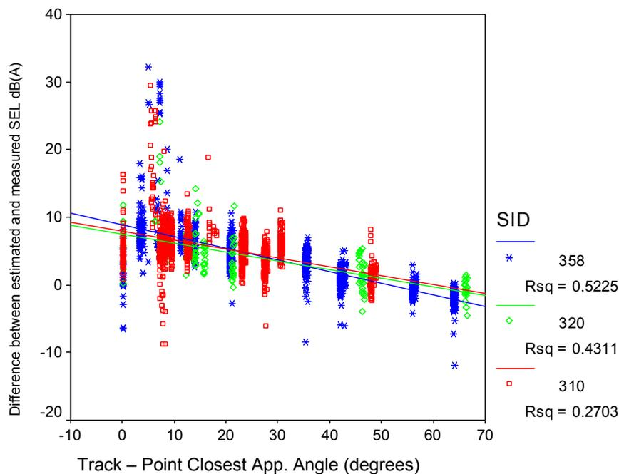
**Figure 11: Measured and estimated SEL differences (separated for each SID – 310, 320, 358) as a function of  $\beta$  angle.**
