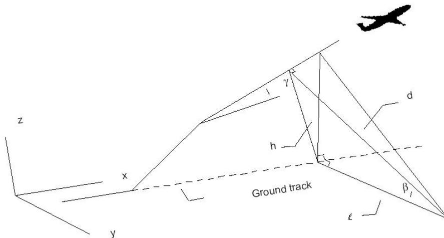
**Figure 10: Representation of noise propagation with respect to trajectory (from ECAC [1])**
