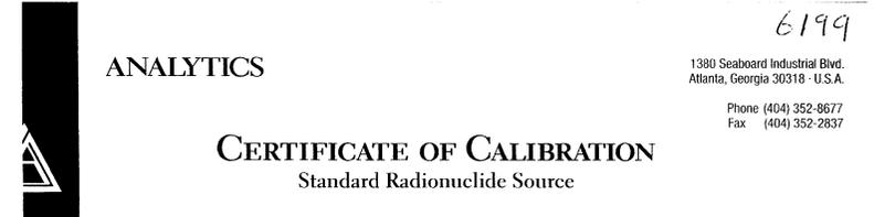
This standard radionuclide source was prepared gravimetrically from calibrated master solutions. The Eu-152 was calibrated by the Department Des Applications Et De La Metrologie Des Rayonnements Ionisants (DAMRI), Paris, France, as Number 25200. All other radionuclides were calibrated in an ion chamber that was calibrated by the National Physical Laboratory, Teddington, U.K., and is directly traceable to national standards.
